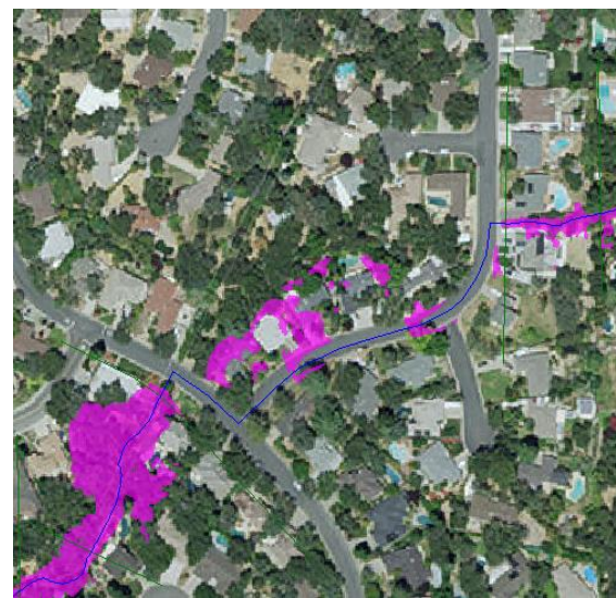
Figure 5: 10 Year Floodplain with Upsized Storm Drain
