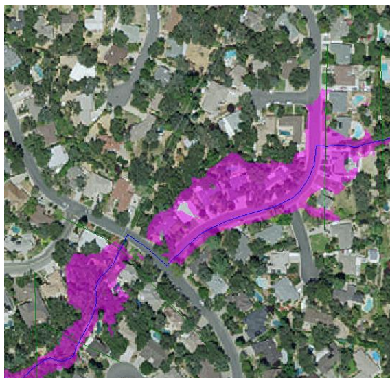
Figure 4: 10 Year Floodplain with Existing Infrastructure
