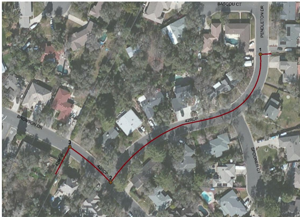
Figure 9: Existing Pendleton Storm Drain
