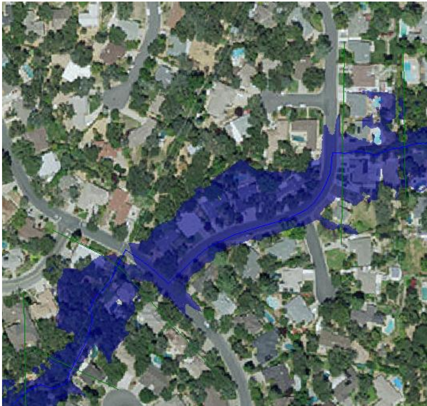
Figure 6: 100 Year Floodplain with Upsized Storm Drain
